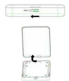
2 Remove the four screws from the printed circuit board, then remove the printed circuit board.
